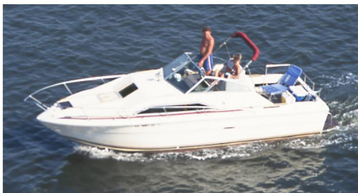
Figure 5: A typical express hull
