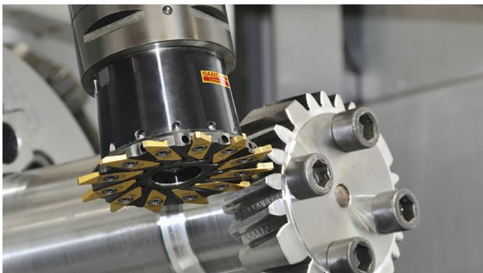
The internal feature of the gear shown in Exhibit 2 was traditionally made with what is called a gear shaper. Using a timed rotation, this machine cuts the gear in a back-and-forth motion. These internal features can now be produced using specific gashing tools on a CNC lathe with live tooling, as shown in Exhibit 4: Spline Milling Head. This has been the latest in technology from the CNC world advancing gear production on a 5 axis CNC Machine from a traditional gear manufacturing machine.
