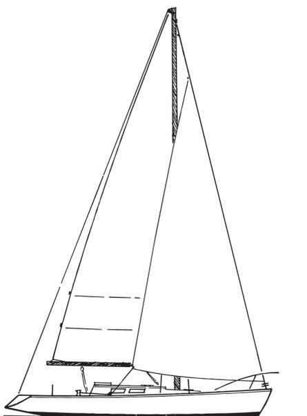
Figure 16: Sloop with masthead rig
