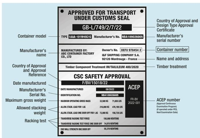
**Figure 2.** Container CSC combined data plate explained | BIC
