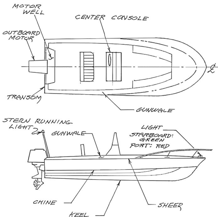
Figure 12: Powerboat terminology: center console runabout
